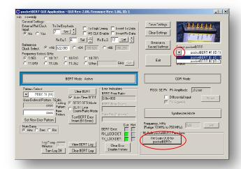
The drop down menu lets you select, modify and monitor a particular unit. If a pB10A is added or removed at a later time, click "Re-Scan USB for pocketBERTs" to update your system settings.
