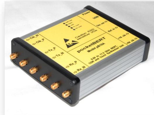
There is no need for an external reference clock as the unit uses an internal programmable clock generator. If needed an external reference clock can be applied.
