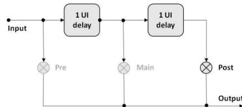
The Pre and Main Tap are factory set and the user has control over the Post-tap to optimize signal fidelity in his transmission path.
